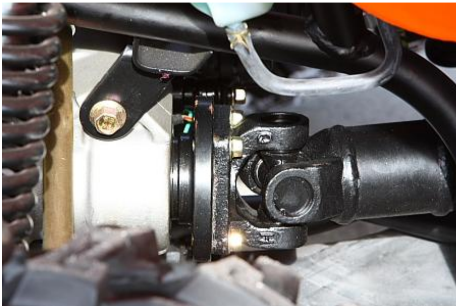
Frame and rear drive-shaft
