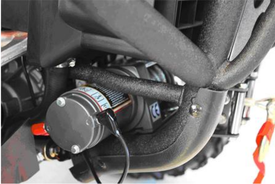
The large capacity winch, mounted underneath the front grill.
