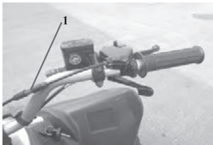
1. Throttle lever free play adjusting bolt
