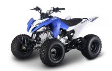
The Rover 125 is a larger 125cc ATV featuring independent front suspension with front and rear disc brakes unlike most drum brake machines on the market. This ATV is loads of fun to ride and the seat is well padded meaning the rider stays comfortable for longer.
