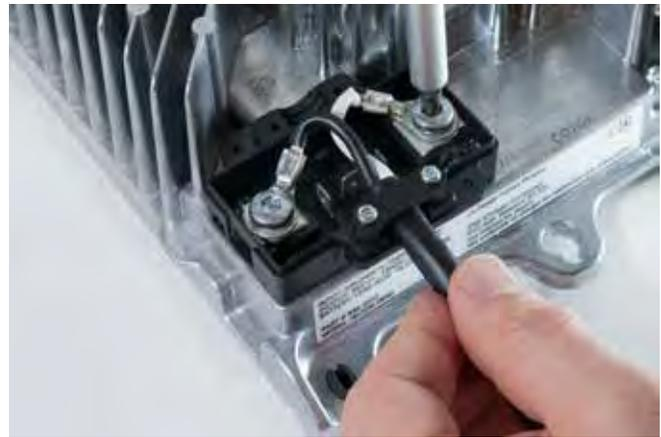
Step 2: Attachment of the DC cable with a Torx T30 screwdriver
