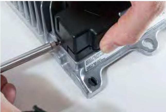
Step 1: Removal of the IC650 DC block cover using a screwdriver.
