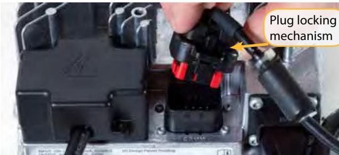
*Insert the TE Connectivity AmpSeal Plug into the Comm fixture with the locking mechanism facing toward the outer edge of the charger.*
