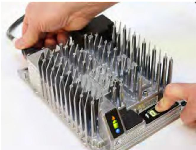
Reconnect AC input while holding the Select Charge Profile Button.
