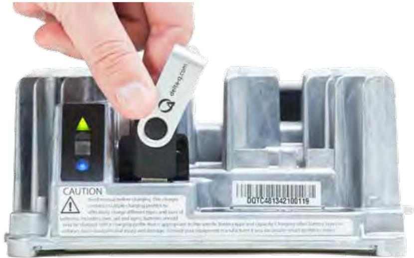
*Insert the USB flash drive to begin the reprogramming process. When complete, the Fault / Error / USB indicator will be solid green as shown.*
