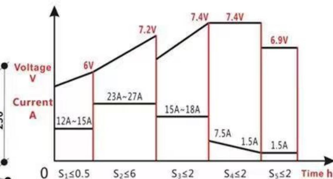
The standard temperature for this charging curve is 25°C
