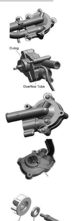
Remove mechanical seal with special tool
