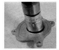
Install bearing with special tool
