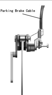
Inspect the brake lines and brake line connections for possible leaks or loose lines.
