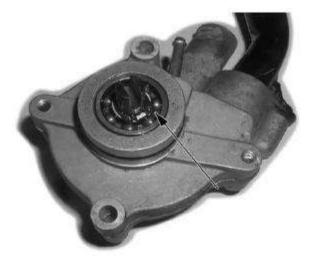
Install new gasket to water pump body;
