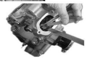
Take out the feeler gauge, measure the clearance. If the clearance is incorrect, repeat the above steps until the proper clearance is obtained. Locknut: 10 N•m
