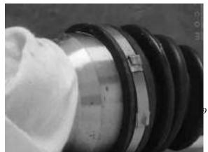
**CAUTION:** It is critical to avoid undue stress on the rubber boots after the drive axle is installed and the vehicle is run. Don't twist the boot, and always set the both ends in designed position.
