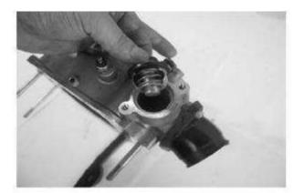
Compress the valve spring and remove valve cotter with tweezers.
