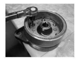
Check starter clutch roller and holder for abnormal wear or damage. Wear or damage:  $\rightarrow$  Replace
